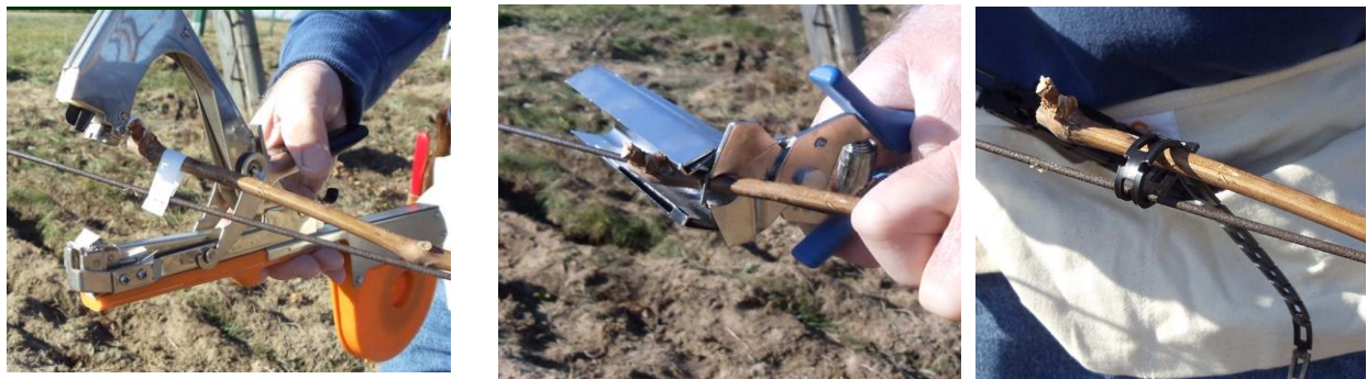
Figure 9: Examples of manual shoot tying tools available. The left-most image uses paper tape, the center image uses metal staples and the right-most image shows a plastic tie.
