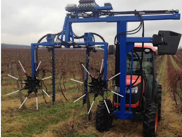
Figure 2: A mechanical pruning system that uses rotary combs to lift the vines and vertical cutters to remove the excess vine.
